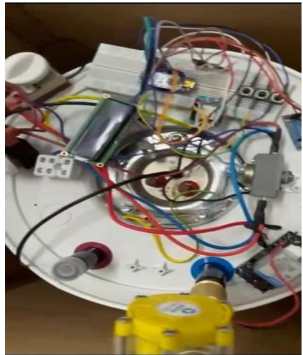
Fig. 11. An assembly of Aqua Sink Pro system
