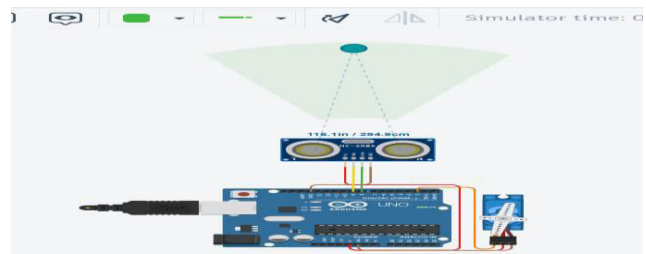
Fig. 9. Ultra Sonic Sensor with Motor
